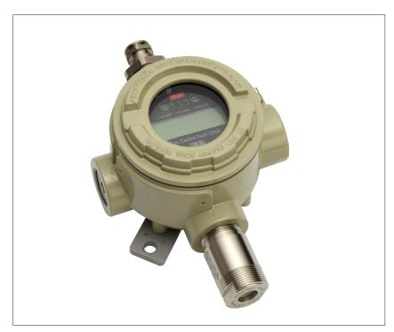
The Heavy Duty gas detection units are used for monitoring and warning of hazardous Ammonia gas concentrations. They are intended for ATEX/ IECEx applications and consists of a robust flame-proof metal enclosure that can be kept closed after wiring, since programming (configuration) is performed by magnetic field to the display via a magnetic pen.Depending on the application, they are available with an electrochemical, a semiconductor or a Pellistor sensor covering a wide range of ppm.
