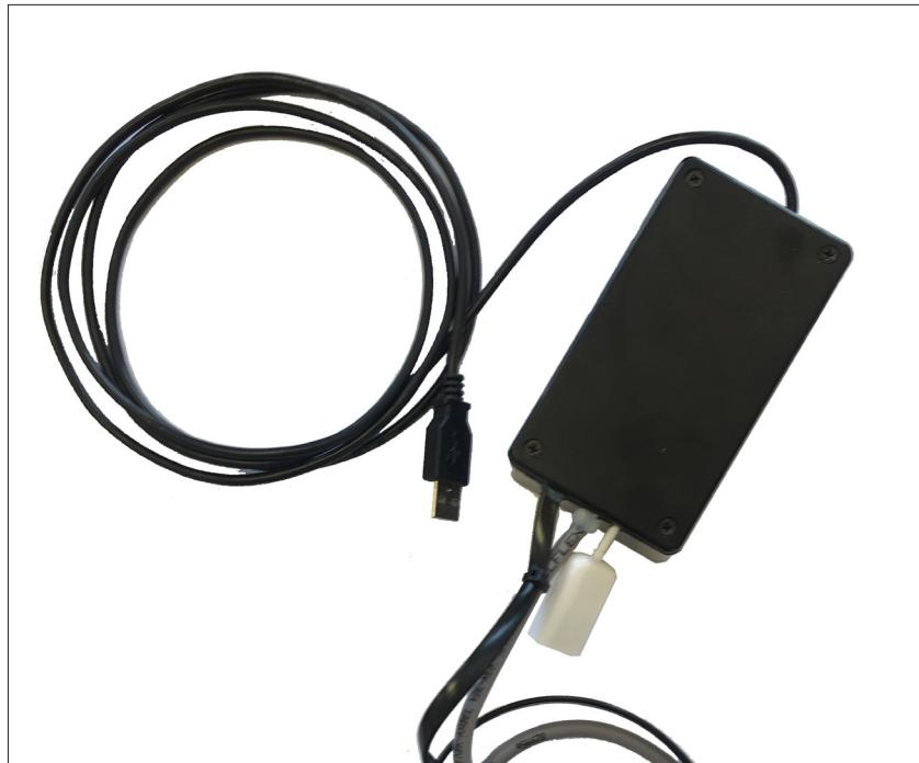
The gas detection PC tool is a menu-driven and stand alone software used for easy Addressing, Parameter setting, Calibration and Data logging of the Basic, Premium and Heavy Duty gas detection units. Furthermore, it handles Parameter setting and Memory Read of the gas detection Controller including peripherals (Expansion module - Warning module). Power for this tool is provided from the PC via the standard USB connection.
