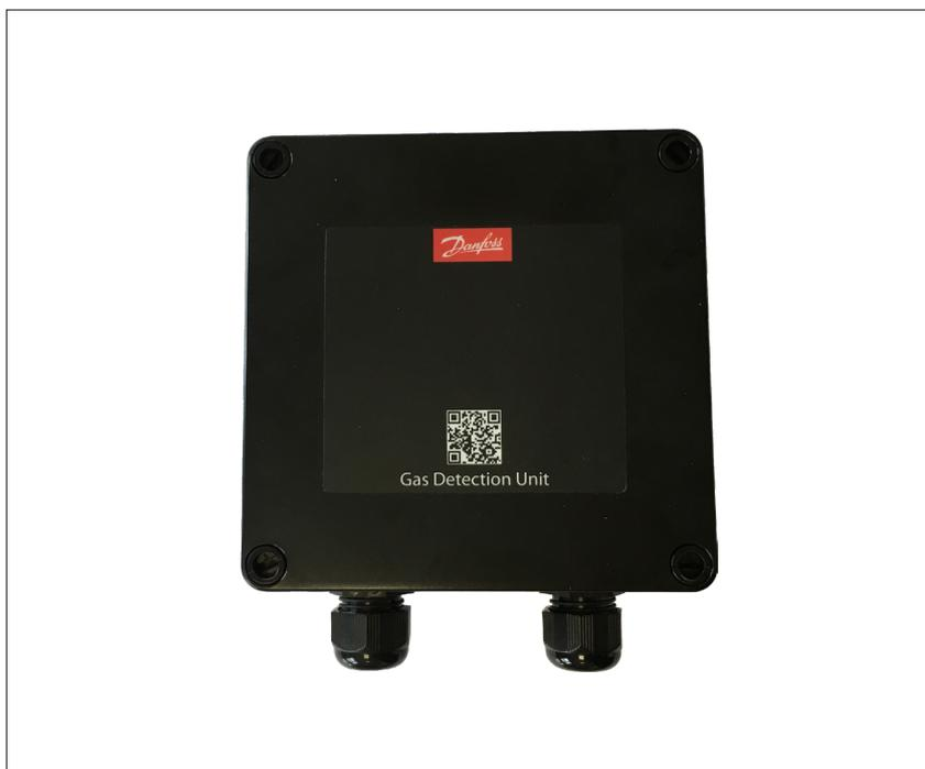
The gas detection warning module is used for increasing safety of a centrally controlled gas detection system by managing the warning/ alarm devices and continuous monitoring the circuiting to the warning/alarm devices. Potential wire breaks or wire interruptions in the alarm device loop will be detected immediately and reported to the central control.
