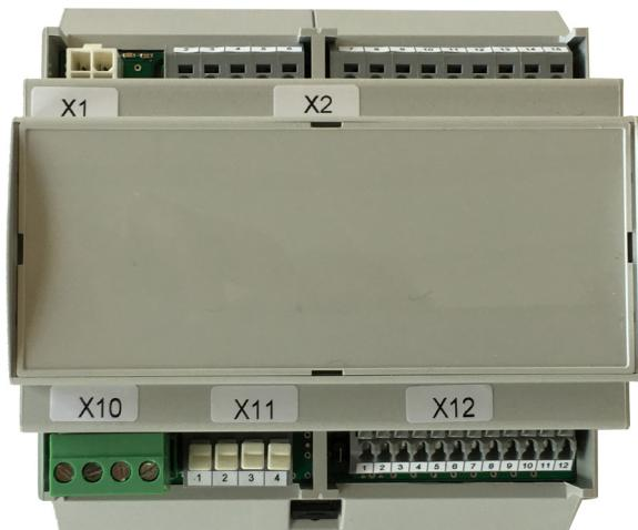
The gas detection Controller Expansion module is used for expansion of the cable coverage in terms of number of fieldbus loops and the total wire length. Each Controller Unit can handle up to 7 Expansion modules allowing 7 additional loops of 900 meters (2953 ft) length available for local Gas Detection Units. Communication between the Controller, the Expansion modules and the Gas Detection Units is done via Analog or RS485 fieldbus.
