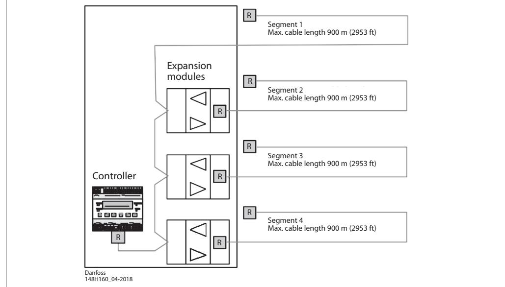
*Expansion modules installation in the field. Resistor R (560 Ohm)*
