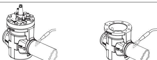
Only for heat controlled welding with no welding debris.
