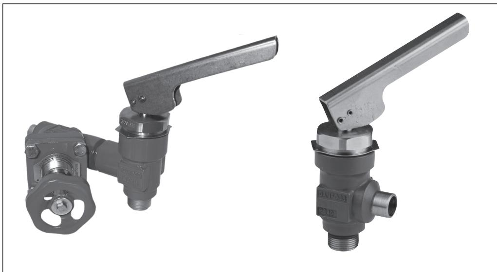
QDV is a quick closing oil drain valve, designed particularly for draining oil from systems containing refrigerant (ammonia) under pressure. The valve will close immediately on release of the handle, thus protecting user and environment against unnecessary refrigerant leaks. The valve should as a rule be installed as illustrated in fig. 1. In order to prevent hydraulic pressure building up
