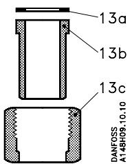
Welding nipple connection for outlet
