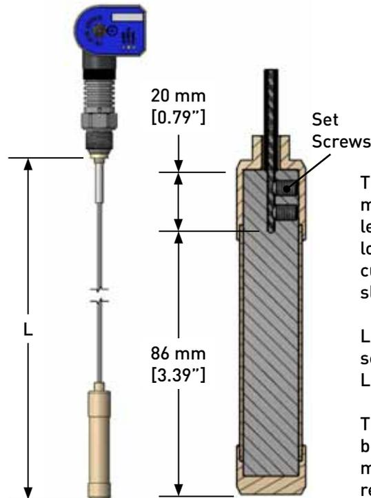
The HBLT-Wire is easily modified to the desired length in the field by loosening the set screws and cutting the wire and teflon sleeve to length.
