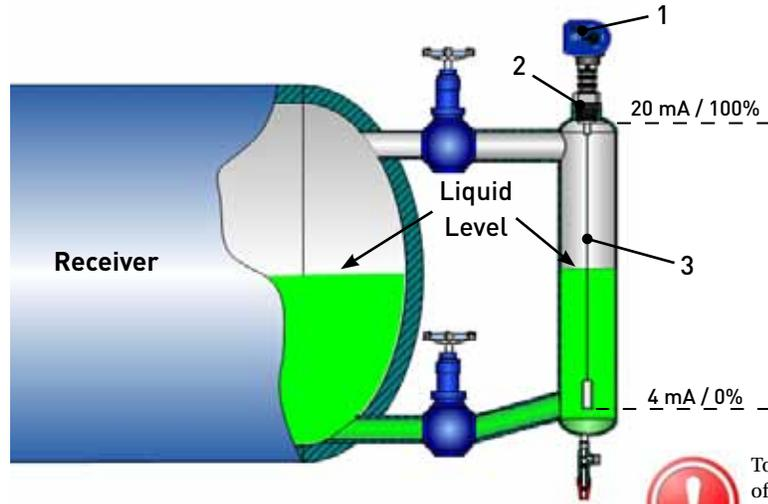
**!** To avoid accumulation of oil in the stand pipe a 10 degree slope on connection pipe is recommended.
