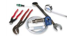
To install the HBLT-wire, you must use a 2.5 mm Allen key, shifting spanner, wire cutter and liquid gasket.
