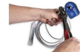
Loosen the electronic part from mechanical part.
